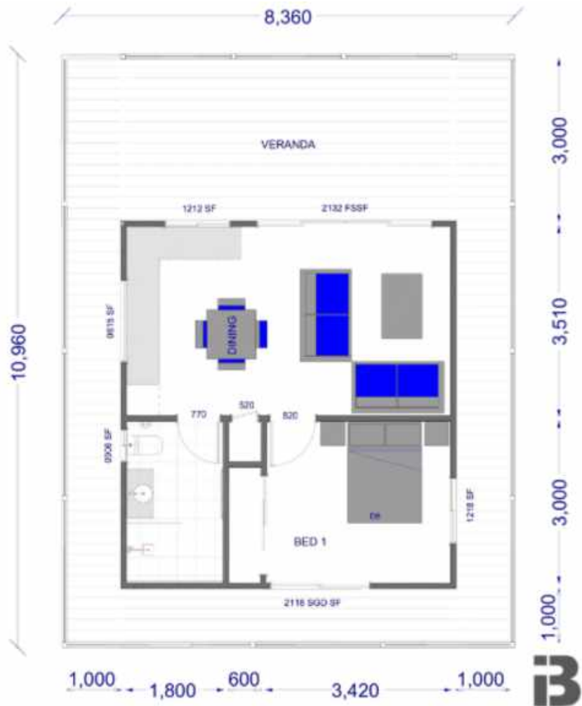
Figure 3.4.12 Layout and measurements of single bedroom cabin (enclosed area: 42.17m 2 , veranda area: 49.44m 2 , Total footprint: 91.61m 2 )
